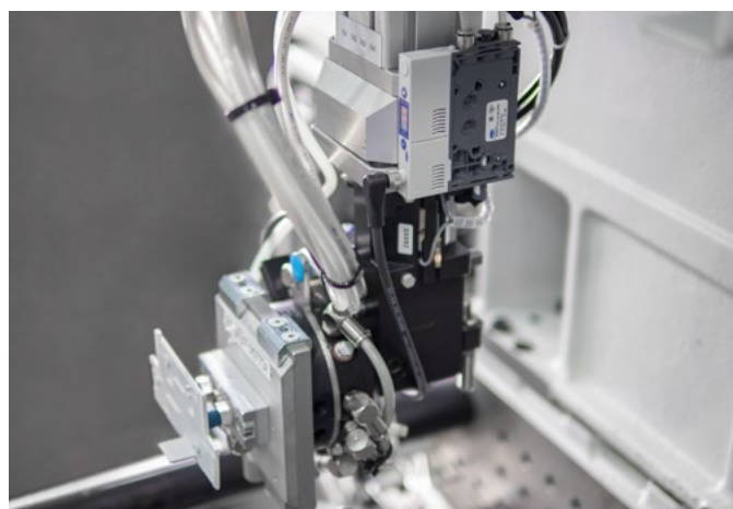
Compact Ejector SCPMc while removing plastic injection moulded parts
